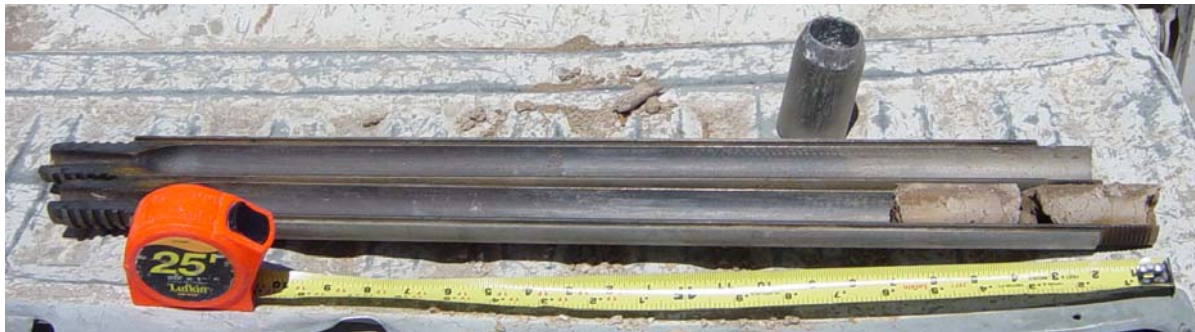
Figure 3-8. Split barrel sampler.
