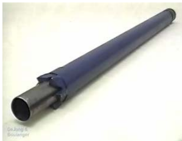
Figure 3-12. Pitcher sampler (FHWA, 1997, 2002b).
