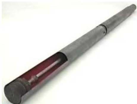
Figure 3-10. Stationary piston sampler schematic (after ASTM D 4700) and photo (FHWA, 2002b).
